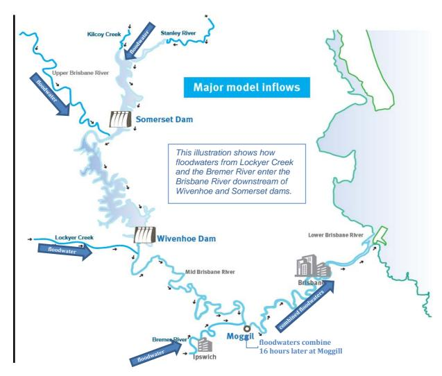
The dam operators measure the floodwaters in the Brisbane River at Moggill as it is the first place where major floodwaters all combine. The dam operators try to avoid the highest releases from Wivenhoe Dam arriving at Moggill at the same time as the highest floodwaters from Lockyer Creek and the Bremer River.
